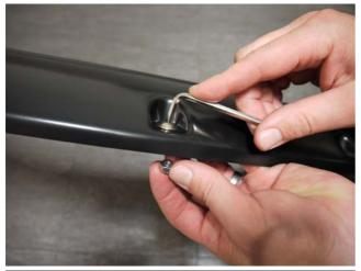
**STEP 9:** Attach 10 bolts to each Fender Flare using a 3/16" Allen key and a 10.0mm wrench/socket. (wrench/socket and Allen key not supplied). Ensure inside of Fender Flares where the rubber seal is attached is clean, using the alcohol wipes provided. Wipe away any residue with a drv clean cloth.
