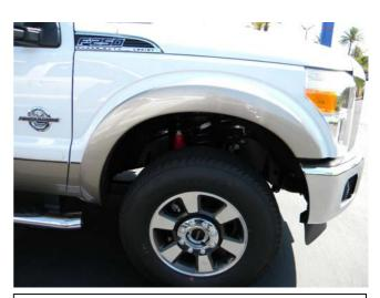
**STEP 6:** Remove all 5.5mm socket head screws and retain for installation of Fender Flares.
