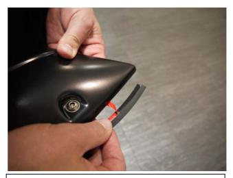
**STEP 10:** Attach the included rubber seal to the Fender Flares. Peel back 2" of the adhesive backing and position on the Fender Flare. Attach the seal to the Fender Flare, peeling back a few inches at a time. Attach rubber seal along all areas the Fender Flare will make contact with the vehicle body.
