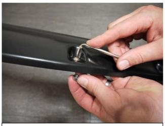
**STEP 1:** Attach 9 bolts to each Fender Flare using a 3/16" Allen key and a 10.0mm wrench/socket. (wrench/socket and Allen key not supplied). Ensure inside of Fender Flares where the rubber seal is attached is clean, using the alcohol wipes provided. Wipe away any residue with a dry clean cloth. For model year 2011 and newer, only 8 bolts are use.
