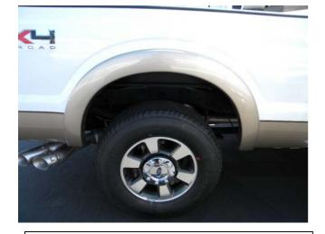
**STEP 11:** Clean the body areas where the Fender Flares will makes contact. Use the supplied alcohol wipe.
