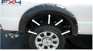
**STEP 12:** Place the Fender Flare onto the vehicle and fit into the correct position following the contours of the body. Use ten (10) of the .6mm clips (five 5 per side) to secure the Fender Flare to the body. Make sure the dimple in the clip securely attaches in the slot on the Fender Flare.
