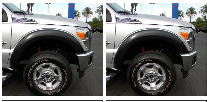
**STEP 7:** Place the Fender Flare onto the vehicle and fit into the correct position following the contours of the body. Ensure the slots in the part align with the holes in the fender from the previously removed 5.5mm socket head screws.
